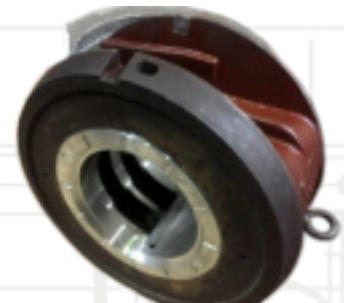
Rebabbiting of White Metal Bearing
